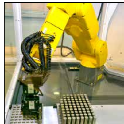
Robotic load and unload of raw materials and finished tools
