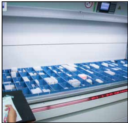
Vertical, barcode controlled inventory storage
